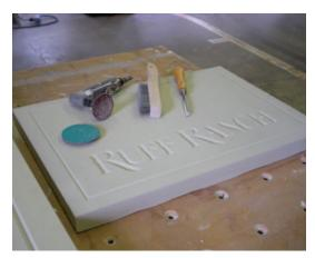
**2. CNC cut border and primary copy, both sides: 30 minutes.** Here you can see the chisel, rotary die grinder and wire brush we used for add the weathered wood grain effect.
